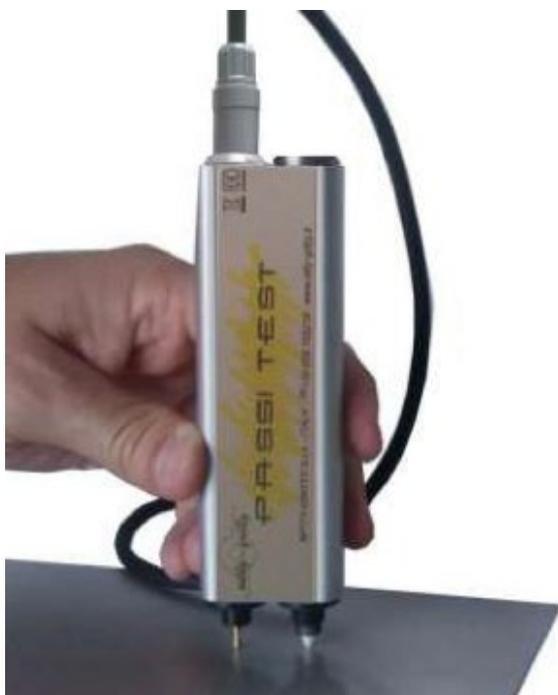
The external unit has a monitor that displays a value related to the nobility of the metal. In the case of stainless steel, this value has a particular range that the meter reads using the “zero” as discriminator: that makes it easy to read even to the inexperienced user, associating a positive value to the “good” passivation status and a negative to “bad” passivation.
